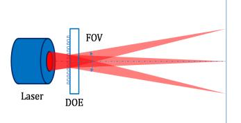
A DOE functions with a laser light source that emits a diffractive pattern. Each DOE pattern is characterized by a specific laser wavelength, focal length and transverse mode. Each laser wavelength will result in a different zero order intensity. The focal length is dependent on the DOE and the object distance which can be adjusted using a collimating lens (CL). The transverse mode will affect the dot shape.
